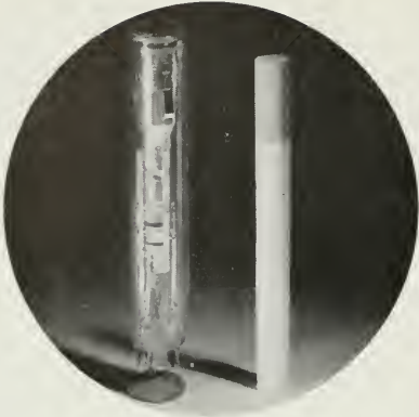
At heart of RCA's new transistorized TV camera is this RCA-developed 1/2-inch Vidicon tube, shown here in comparison with a king-size cigarette. Tube is now being produced in sample quantities.
